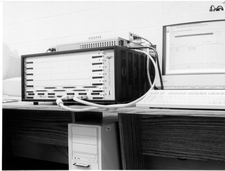
Figure 5: Photograph of IKOS Virtuallogic SLI logic emulator.
