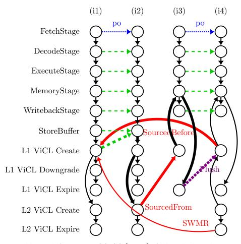
Figure 6.11:  $\mu$ hb graph for mp on TSO-CC [EN14]. Although the coherence protocol does not eagerly invalidate any sharers of **x** before allowing (i1) to perform, the necessary orderings are enforced by (i3) flushing the cache upon taking a cache miss.
