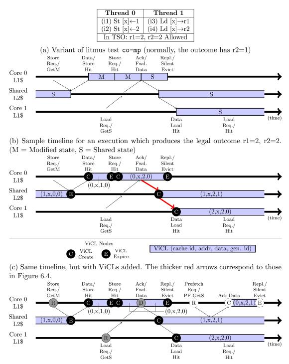
Always Enumerated Enumerated as Needed Not Enumerated ViCL ViCL ViCL \$ Line \$ Line ViCL \$ Line  $(\bigcirc) \stackrel{\text{VICL}}{\text{Create}}$ (R)(D)(E)  $\mathbf{R}$ CExpire Request Downgrade Expire Request Create
