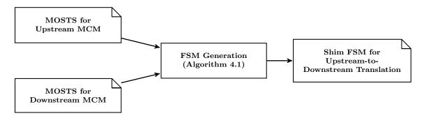
Figure 4.4: Shim FSM generation process overview
