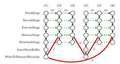
(c) Cyclic (and hence unobservable)  $\mu hb$  graph for an execution in which all reads skip the store buffer and access memory
