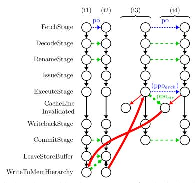
(a) Speculative load reordering: although  $ppo_{arch}$  is not enforced, a legal replacement  $ppo_{slr}$  is enforced, and it completes the cycle.
