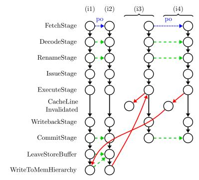
(a) Pipeline bug shown via the mp litmus test. The lack of a cycle indicates that the behavior is (erroneously) observable.
