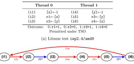
(b) Architecture-level analysis. Even though there is a cycle, there is no cycle involving the subsets in Figure 5.1b, and so the outcome is permitted.
