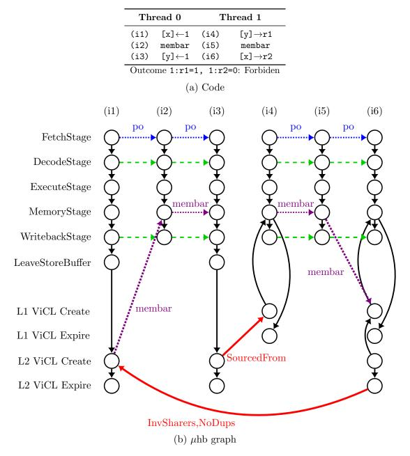
Figure 6.9: Modified mp [ABD<sup>+</sup>15] on a hypothetical GPU with no-allocate-on-write and no SWMR guarantee. In particular, the thread 1 fence does not enforce the load $\rightarrow$ load ordering, and so there is no cycle.
