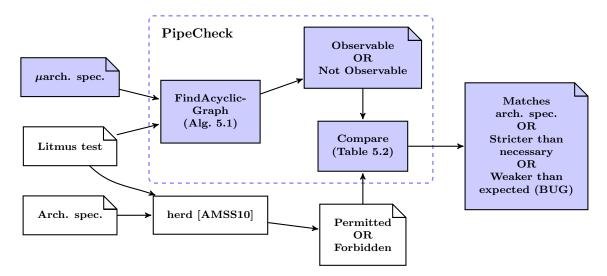
Figure 5.7: PipeCheck block diagram and toolflow. Pre-existing components are shown in white; shaded components were created for PipeCheck.
