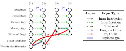
(b) In this example, the preserved program order (**ppo**) edges are discarded as an architecture-level assumption, and the model verifies that enforcement required by those edges is instead enforced by some combination of  $\mu$ hb edges.
