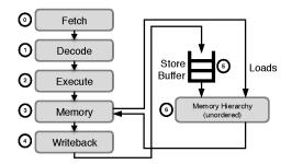
(a) Classic five stage RISC Pipeline plus a FIFO store buffer and an unordered memory system. This pipeline example recurs throughout this chapter.
