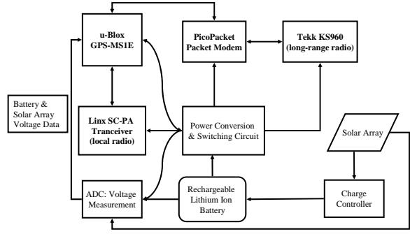
**Figure 5: Block diagram of ZebraNet node design.**
