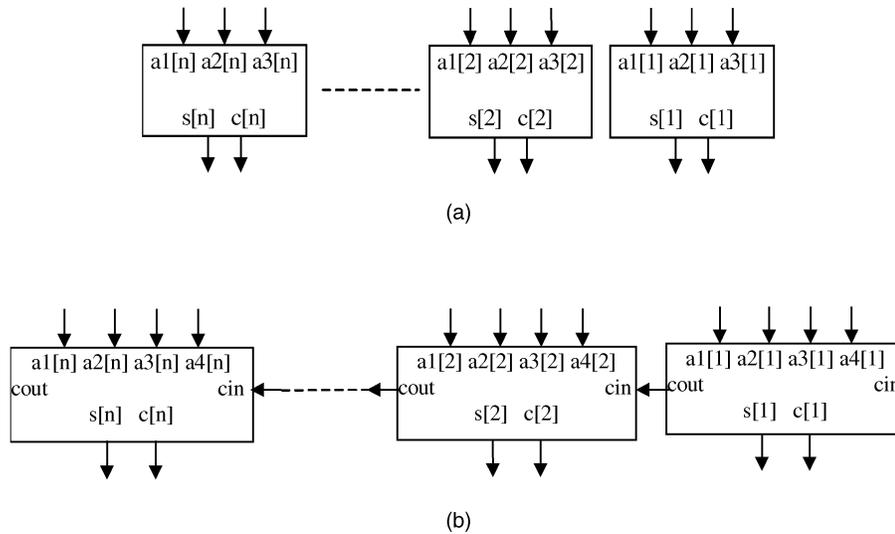
Fig. 1. (a) An array of  $n$  3-2 adders. (b) An array of  $n$  4-2 adders.
