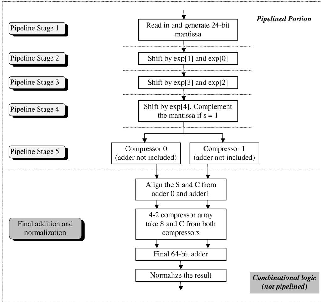
Fig. 7. Floating-point accumulator with compiler-managed overflow avoidance pipelining scheme.
