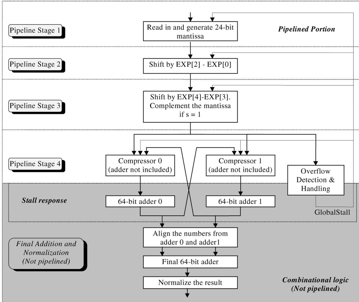
Fig. 6. Floating-point accumulator pipelining scheme.
