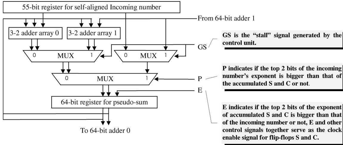
Fig. 5. Compressor design (compressor-0).
