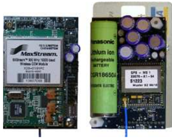
Figure 4: Photo of a ZebraNet node (2" x 3" x 1.25"). The left card includes the radio and the right card includes the GPS chip and the battery. A credit card is included in the picture for scale.
