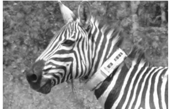
Figure 10: Plains Zebra at Sweetwaters Game Preserve with ZebraNet collar. The collar is made of a white butyl belting material. The darker spots visible on the upper half of the collar are the solar modules which lie between the two layers of butyl belting, with openings exposed to allow sunlight in.
