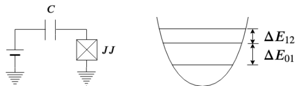
Fig. 17. Left: an LC circuit. In SC LC circuits, normal current becomes SC current. Right: the energy potential of a harmonic oscillator. In QHOs like the SC LC circuits, the system energy becomes equally spaced discrete values. The plotted two levels are the ground state and the first excited state.
