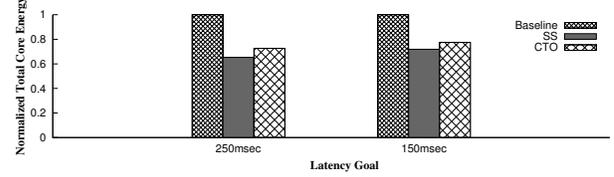
**Figure 6.** Effect of latency goal on total core energy. With the lower latency goal, total core energy consumptions increase since the idle energy increase with the more number of ON cores. The increase in idle energy increases the energy spent by SS around 10% and CTO around 6%.
