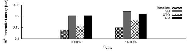
**Figure 5.** Effect of contention on 75<sup>th</sup> percentile latency with different core count management schemes. Latency is increased in all schemes under contention. The increase in CTO is higher than the increase in SS because more cores can be busy at the same time, hence are affected by the contention more. The increase in RR is higher than the baseline case because of the similar reason.
