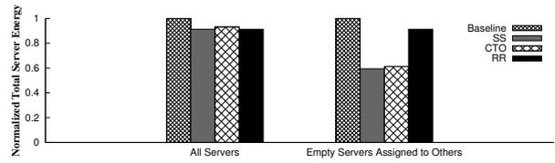
**Figure 8.** Normalized total server energy when all active servers are dedicated to the main application and when the empty servers are assigned to other jobs. Making use of empty servers results in 41% decrease in energy with SS method.
