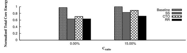
**Figure 4.** Effect of contention on total core energy with different core count management schemes. Energy gains obtained by different schemes decreased by the contention in different amounts. Increase in total core energy consumption with RR scheme is around 13% while in SS, this increase is almost 30%.
