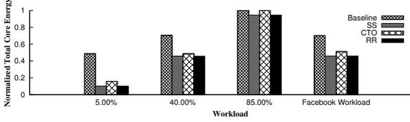
**Figure 2.** Normalized total core energy at different workload levels. Although energy saving with SS is 35% compare to baseline case under Facebook workload, it can reach up to 80% when load rate is 5%.
