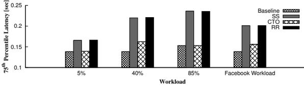
**Figure 3.** 75<sup>th</sup> percentile latency at different workload levels with different techniques. All techniques manage to ensure the latency goal of 250 msec.
