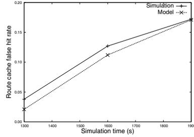
**Figure 8. Comparison of  $\pi_f$  changes detection (simulation vs. model).** The epoch length is 300s and the packet injection rate is 2pkts/s.
