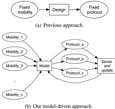
**Figure 1. A model-driven adaptive routing architecture.** Our approach can be applied to different protocols with every protocol customized on-the-fly to mobility changes.
