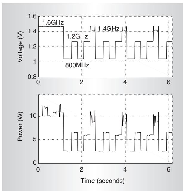
Figure 5. Partial traces of CPU voltage and power for SPEC benchmark 173.applu running with RDO.
