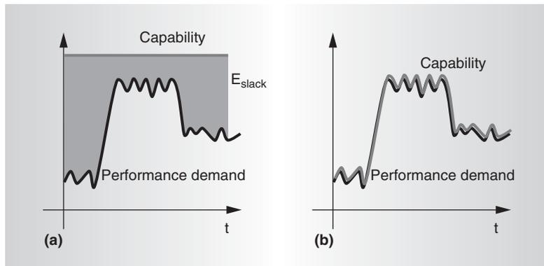
Figure 1. For a processor, online dynamic voltage and frequency scaling aims to scale frequency to match varying performance demand. Without DVFS (a), energy waste ( $E_{\text{slack}}$ ) occurs (shaded area), but a perfect DVFS control scheme (b) can result in a perfect match between domain-execution capability and demand.
