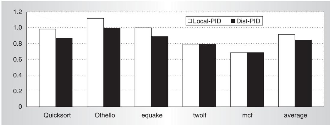
Figure 6. Energy-delay product with local-PID and dist-PID. We normalized both schemes against a baseline (EDP of 1.0) in which a processor shuts off the tile when its task queue is waiting for threads. In all cases, dist-PID equaled or outperformed local-PID.
