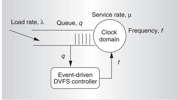
Figure 2. Single-queue model for a clock domain with input queue  $q$ . The circle represents the clock domain being considered, such as a floating-point functional unit. The domain has frequency  $f$  and an execution capability or service rate,  $\mu$ , a function of  $f$ . The performance demand is  $\lambda$ , and the queue has finite size.
