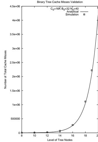
Figure 9: Validation of Binary Tree:
