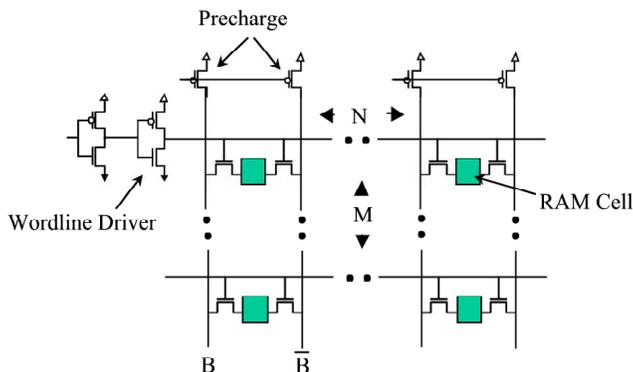
Fig. 3. RAM array schematic. Transistor-level schematics like the one shown here are used to create mathematical equations that estimate internal node switching capacitance.
