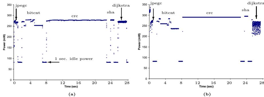
Fig. 7. Measured (left) and simulated (right) power consumption for five MiBench benchmarks. For this set of benchmark the maximum error is 11% (JPEG) and the minimum is 3.66% (Bitcount). Benchmarks are separated by a 1 second delay seen as 80mW idle power.
