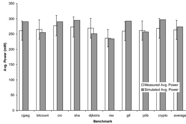
Fig. 10. Average power consumption for MiBench and open CLDC Java benchmarks. 12 percent error bars are shown.
