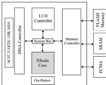
Fig. 2. Processor block diagram. The Intel XScale core is surrounded by support functional units that contribute to the processor’s overall power consumption. Not all peripheral units are shown in this figure.
