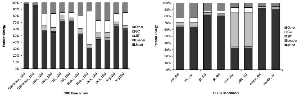
Fig. 12. Energy distribution among five JVM components for CDC (left) and CLDC (right) Java applications. The suffix attached to the benchmark name specifies the maximum heap size used by the JVM.
