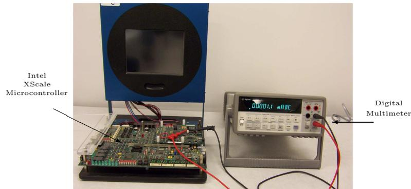
Fig. 4. Physical measurements setup. The Agilent 34401A Digital Multimeter (DMM) is used to sample current consumption of the Intel PXA255 CPU. High sampling speeds are achieved through a GPIB connection between the DMM and a host PC.
