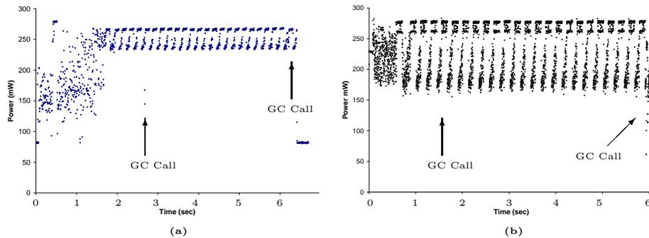
Fig. 8. Measured (left) and simulated (right) power consumption for REX. The start of CLDC benchmarks is characterized by very varied power behavior which corresponds to JVM initialization.
