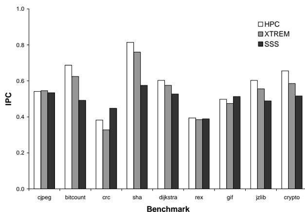
Fig. 6. Comparison between simulated and hardware-measured IPC performance for a set of MiBench and open CLDC benchmarks.
