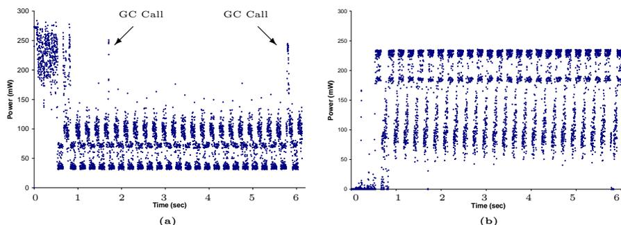
Fig. 14. Simulated power consumption of the JVM system (left) and JITted code (right) for REX
