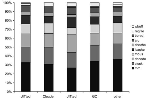
Fig. 13. Functional-unit energy breakdown of JVM components for `javac` with 16M maximum heap size.
