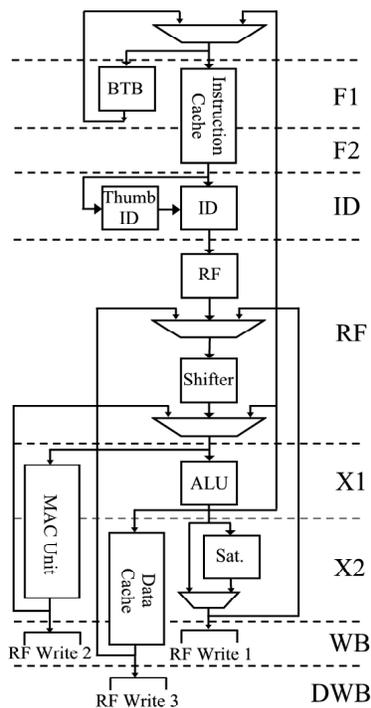
Fig. 1. Block diagram of the Intel XScale microarchitecture pipeline.
