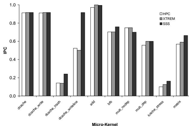
Fig. 5. IPC comparison for stressmarks as reported by XTREM, ARM-SimpleScalar (SSS) and Hardware Performance Counters (HPC). XTREM simulates adequately many aspects of the Intel XScale microarchitecture.
