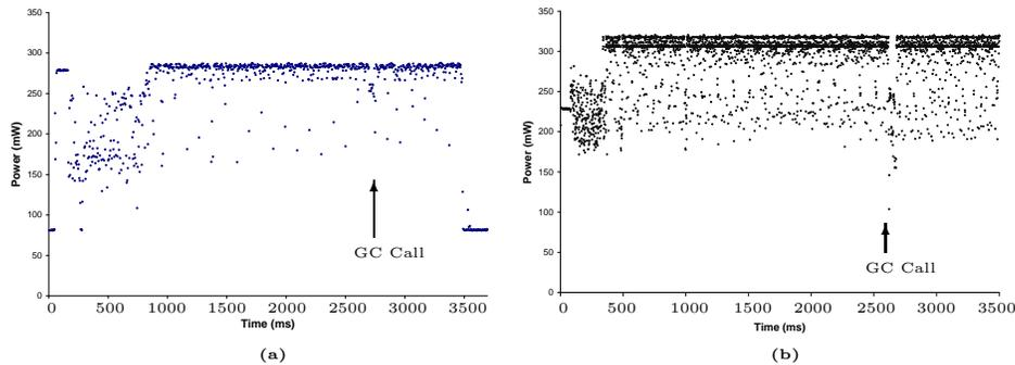
Fig. 9. Measured (left) and simulated (right) power behavior for GIF. A call to garbage collection creates a brief power drop around 2600ms.
