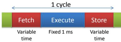
**Figure 3:** The execution sequence of our computer architecture consists of a sequence of variable-length cycles. Every cycle fetches, executes in a SIMD fashion, and stores a number of operand qubits. Although the SIMD operation time remains constant, the operand transportation times vary from cycle to cycle with the number of operands to transfer.
