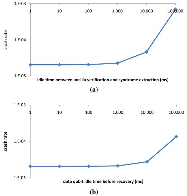
**Figure 10:** (a) Verified ancilla qubits may idle in memory for up to 100 ms (roughly 100 2-qubit physical operation cycles) without significantly impacting the crash rate. (b) Likewise, data qubits may idle in memory for 100-1,000 ms between successive error recoveries.
