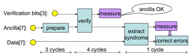
**Figure 9:** The simplest error recovery process: prepare the ancilla block to a specific encoded state; verify that the state is free of X errors; and extract a syndrome by interacting the ancilla with the data block. The ancilla is then measured and decoded via classical processing to determine a syndrome and the proper corrective procedure for the data block. The times listed are in terms of 2-qubit operation cycles, which are roughly 1 ms each for the eSHe QC.
